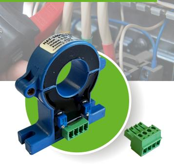
To transfer the measured AC current data, the **VT407 AC converter** is used. It is an analog plug-and-play device that connects to any available analog port on a Vutlan monitoring unit. Providing real-time data on current consumption and enabling the system to react to overcurrent situations or electrical failures.
