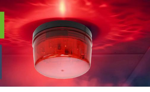
The **VT105 LED strobe light** is a 12V DC device designed to provide flashing light alerts for warnings and alarms. It connects to the 12V DC, 0.25A electronic relay output of Vutlan monitoring systems, offering a visual notification in case of triggered alarm events.
