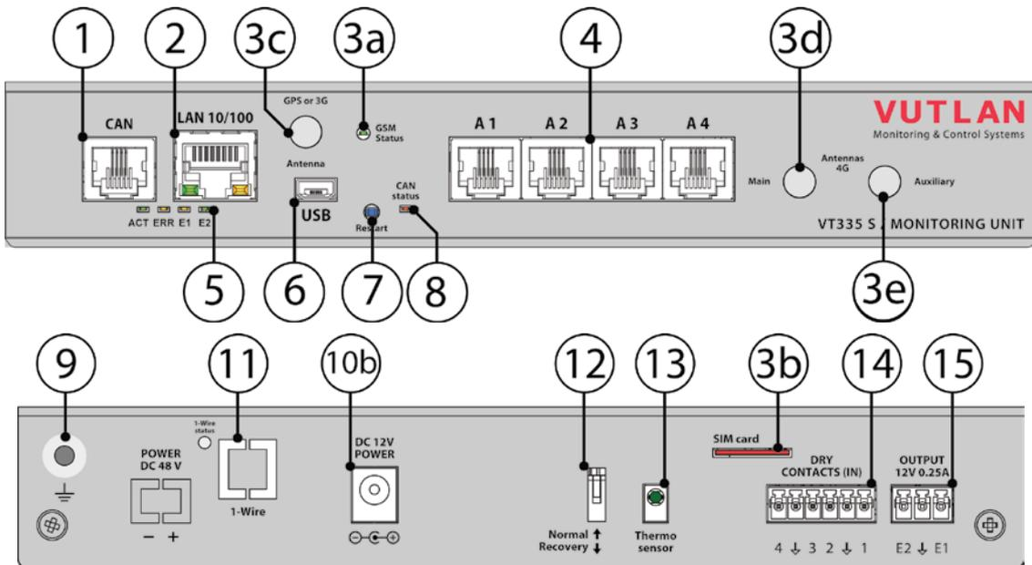
1. "CAN" - digital connector RJ12 for the connection of CAN sensors and CAN extensions on a CAN bus, with auto-sensing.
