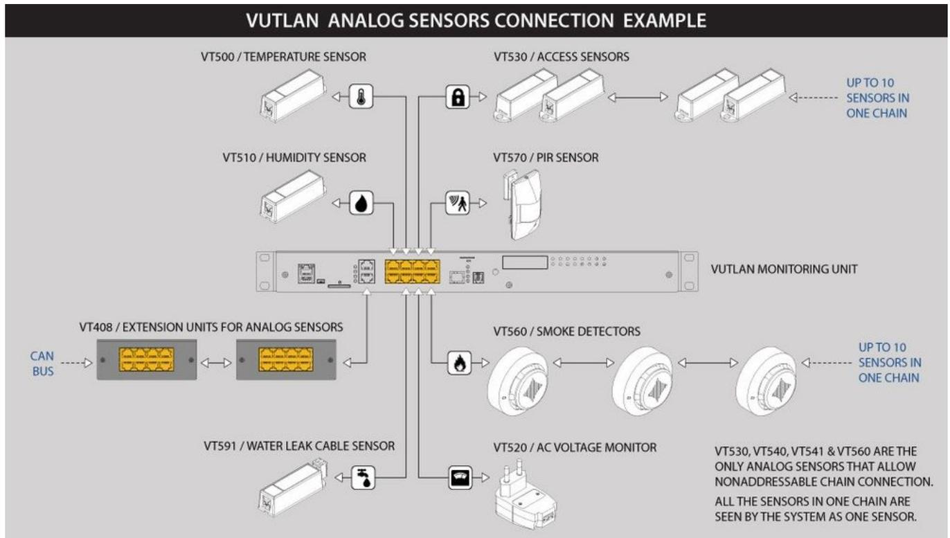
If strong electromagnetic interference is present, we recommend using a 3-pair cable CAN FTP for sensor connection!
